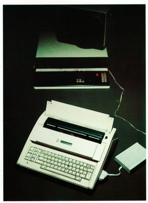
The connection of interface boxes for Commodore/Centronics, V.24 (EIA RS 232 C) and other modules at the user's option is possible through the system interface of the typewriter. So the Erika 3005 electronic can be used as a calligraphic printer for home and personal computers.
